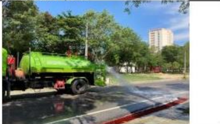
Example of Water Recycling Program, the treated water from aeration pond to clean the streets of the university to reduce PM.2.5 dust values.
